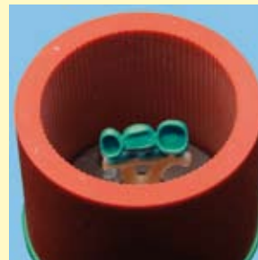
The model is invested in investment material using the thermopress 400 investment ring system.
